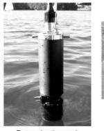
Determination and quantification of up to 5 different algae classes
