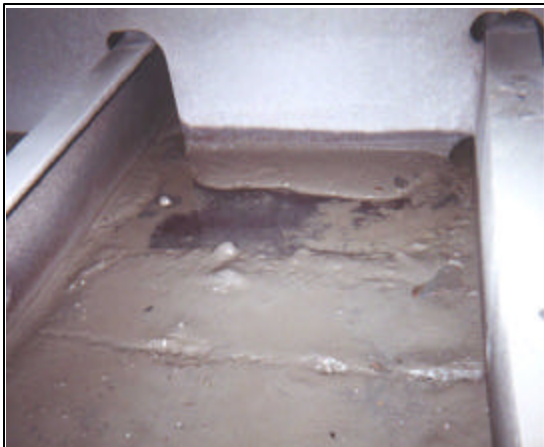
Residual mud in the bottom of a ballast tank on a transoceanic vessel in the Great Lakes during 2001. (Great Lakes NOBOB Project Team)
